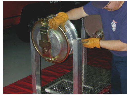
The dome lids themselves rotate for easy filling with water and can be secured at numerous angles to recreate roll-over angles.
